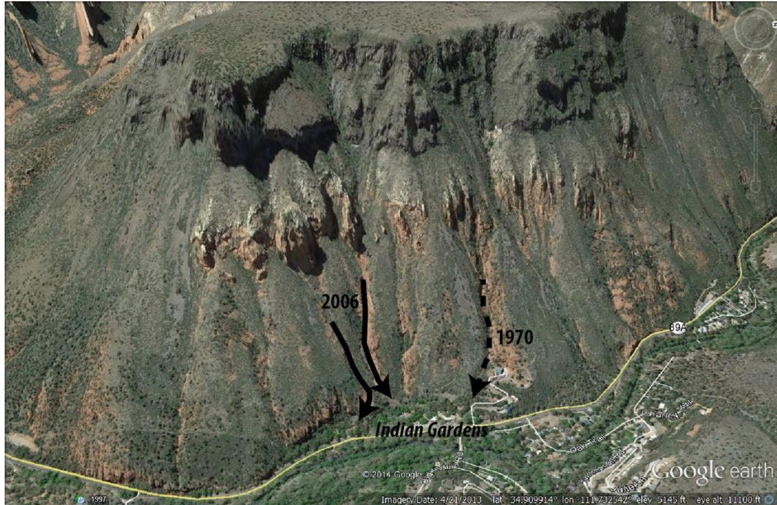
**Figure D1-14: Aerial image of Oak Creek Canyon and Indian Gardens. Debris flows occurred in very steep, small watersheds during the extreme precipitation event of 5 September 1970, and during monsoon storms after the Brins Fire. Base image is from Google Earth.**
