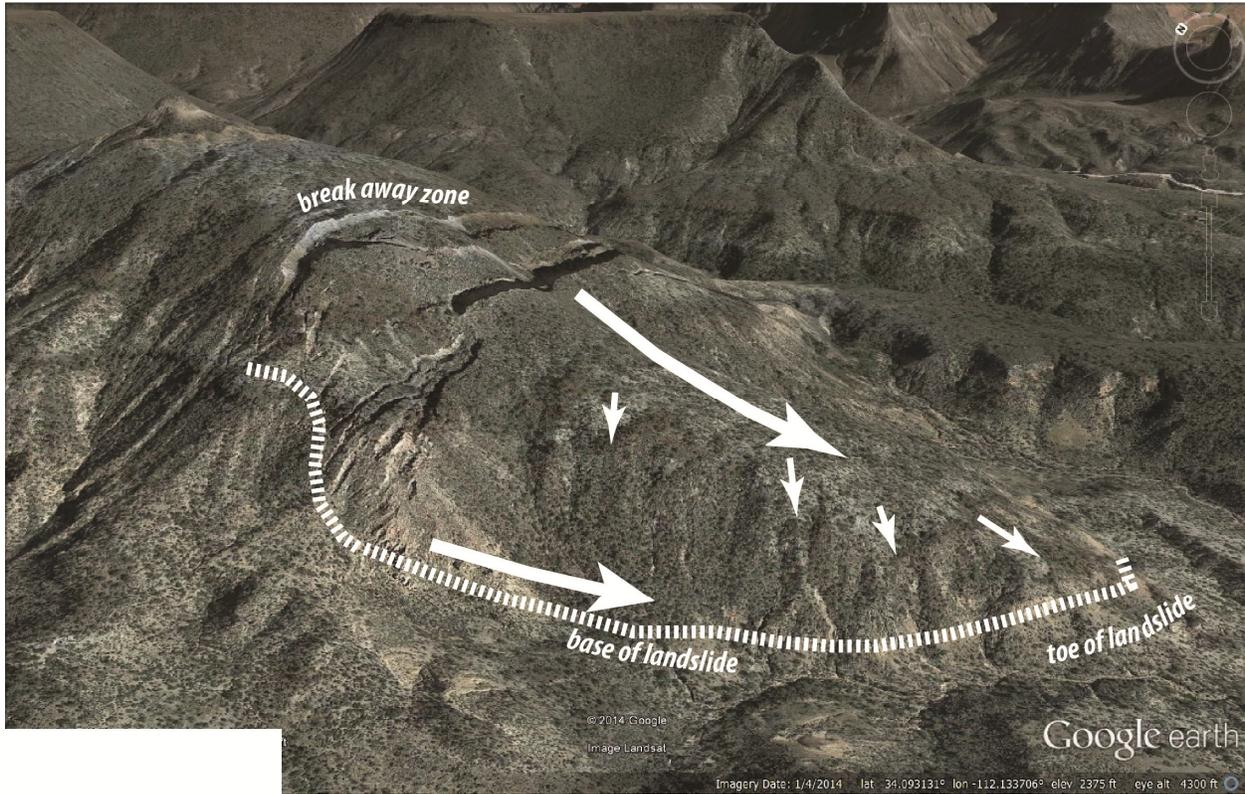
**Figure D1-2. Diagram of the BCC landslide as seen from a southwest perspective. The area on the ridge above the headwall fractures apparently is stable; the landslide mass is moving slowly or intermittently to the south over a clay-rich sedimentary layers. Base image is from Google Earth.**
